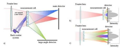
Figure 2. a) The basic outline of ANALYSETTE 22 model with an inverse Fourier optic, b) the measuring cell position for small particle and c) the measuring cell position for large particles [5].
