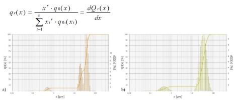
Figure 4. Measurements of copper matrix composite a) poor and b) good result.
